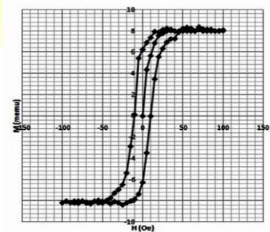
FIGURE 10. CoFeB Sputtered layer (6nm)
