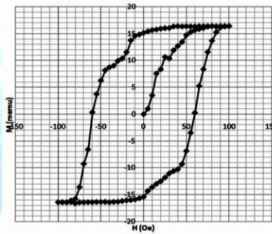
FIGURE 9. CoFe Bi layer (6nm)
