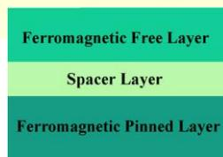
FIGURE 1. Basic structure of MTJ
